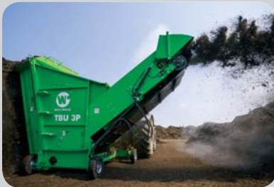
...► TBU in action: Restacking of trapezoidal heaps up to 3 meters with 0,5 km/h more
