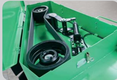
...► The TBU 3P is equipped with a low-maintenance belt drive.
